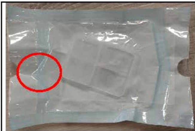
Figure 3- Aural Ventilation Tube present Primary Packaging with defect highlighted in red
